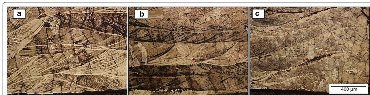
**Fig. 5** Optical micrographs at equivalent locations corresponding to different energy density specimens **a**  $7.4 \text{ MJ in}^{-3}$  ( $\sim 448 \text{ kJ cm}^{-3}$ ), **b**  $6.04 \text{ MJ in}^{-3}$  ( $\sim 369 \text{ kJ cm}^{-3}$ ) **c**  $4.15 \text{ MJ in}^{-3}$  ( $\sim 253 \text{ kJ cm}^{-3}$ )
