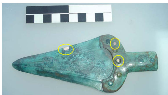
Figure 2 Pugnale da Ripatransone: an example of patina abrasion for measurement- purpose can be seen; the abraded spots are enhanced by yellow circles.
