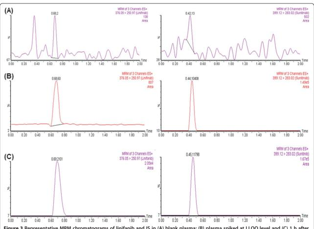
Figure 3 Representative MRM chromatograms of linifanib and IS in (A) blank plasma; (B) plasma spiked at LLOQ level and (C) 1 h after oral administration of linifanib 5 mg/kg in rat.
