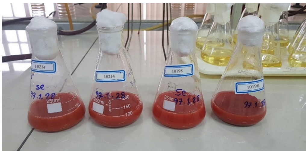
Fig. 1 Color change of the culture from light yellow to red, indicating the biosynthesis of SeNPs
