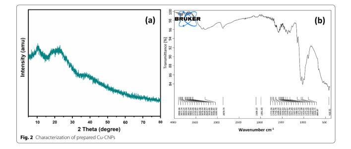
The XRD spectrum showed that the prepared Cu-CNPs had the cubic-crystalline structure, and the corresponding planes were matched with the JCPDS file number (JCPDS NO: 05-0061) [29]. The average crystalline size was calculated by using simple Debye–Schere's formula:
