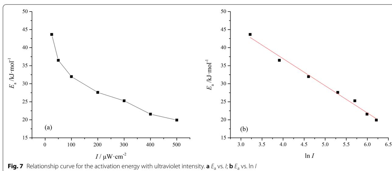
**Fig. 7** Relationship curve for the activation energy with ultraviolet intensity. **a**  $E_a$  vs.  $I$ ; **b**  $E_a$  vs.  $\ln I$ **Table 4** The effect of varying ultraviolet intensity on the quantum yield ( $\Phi$ ) of 1,3-butadiene
