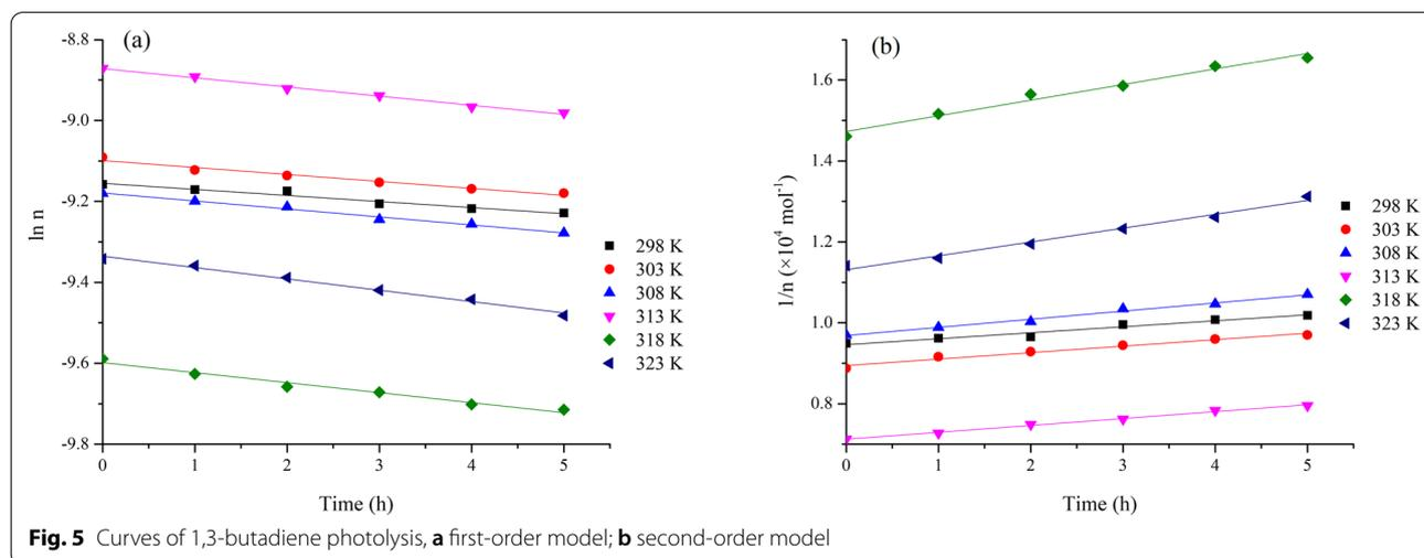
**Fig. 5** Curves of 1,3-butadiene photolysis, **a** first-order model; **b** second-order model
