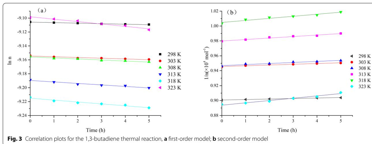
**Fig. 3** Correlation plots for the 1,3-butadiene thermal reaction, **a** first-order model; **b** second-order model
