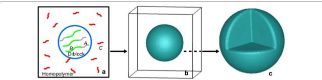
**Fig. 1** a A simulation box contains a diblock copolymer A–B and a homopolymer C. **b** A spherical domain that comprises of a diblock copolymer A4B8 after a domain confinement calculation was performed. The homopolymer that occupies the rest of the simulation box is not shown here. **c** A cut-through of the sphere
