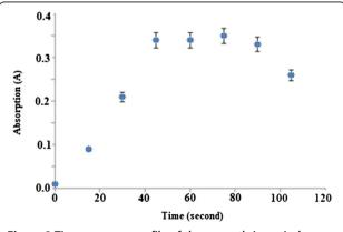
Figure 8 Time response profile of the permethrin optical sensor. Permethrin concentration: 100.0  $\mu$ M; concentration of Gibbs reagent: 1.0 M; pH: 11.0.
