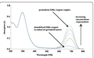
Figure 3 Gibbs reagent absorption spectrum of the absorbed film nafion/sol–gel with permethrin concentrations of 0.0–150.0  $\mu$ M and pH 9.0.
