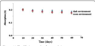
**Figure 11** The lifetime study of permethrin sensor response. Permethrin concentration: 50.0  $\mu$ M; concentration of Gibbs reagent: 1.0 M; pH: 11.0.
