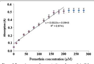
Figure 9 Dynamic range of concentrations of permethrin (0.0–300.0  $\mu$ M) with Gibbs reagent 1.0 M at pH 11.0.
