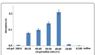
Figure 4 Effects of the nafion/sol–gel silicate ratio towards chemical sensor response. Permethrin concentration: 50.0  $\mu$ M; concentration of Gibbs reagent: 1.0 M; pH: 9.0.
