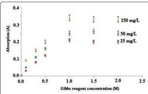
Figure 6 Effects of concentration of Gibbs reagent on chemical sensor response. Permethrin concentrations: 25.0, 50.0, and 100.0  $\mu$ M; pH: 11.0.
