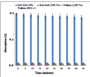
**Figure 7 Leaching study on chemical sensor response.** Permethrin concentration: 50.0  $\mu$ M; concentration of Gibbs reagent: 1.0 M; pH: 11.0.
