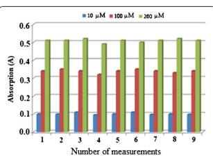
Figure 10 Reproducibility study of permethrin optical sensor. Permethrin concentrations: 10, 100, and 200  $\mu$ M; concentration of Gibbs reagent: 1 M; pH: 11.0.
